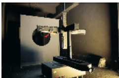
Horizontal Light Distribution Test
